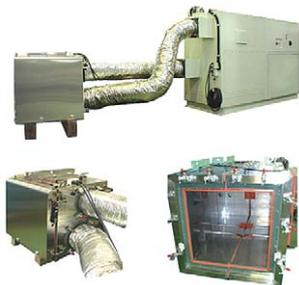
It can be used for development and evaluation of engines and motors for automobiles. The testing equipment is flexible in which the chamber can be fabricated according to the shape of the engine or motor connected to a dynamometer and supplies air conditioned air to the chamber at a remote area using a duct.
